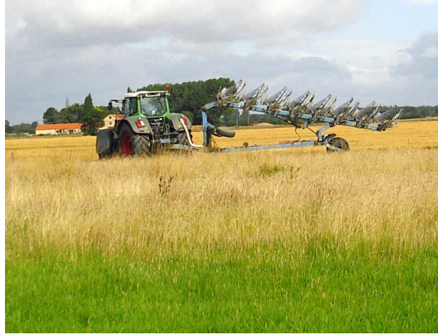
Fig. 3.4 .1 300hp Tractor and 8 furrow plough turning at the edge of the garden only 50 metres from the measuring site
